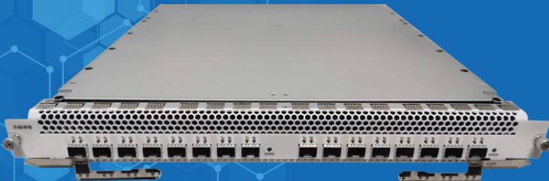
With professional L2-7 traffic generation and analysis capabilities, X2-10G multi-rate test module supports large-scale routing and switch protocols and traffic simulation, and benchmark tests(such as RFC2544/RFC2889/RFC3918), function tests, performance tests, long-term stability and reliability tests for ultra high-density 10GE network equipment.
